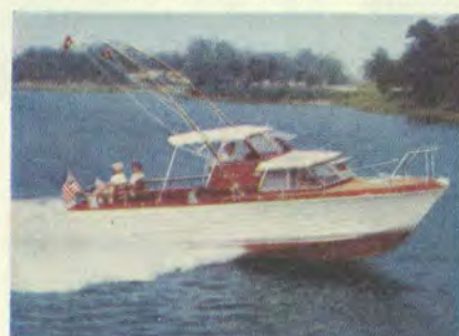
NEW OWENS "29" SEA SKIFF SPORT FISHERMAN—Lapstrake-planked hullsides and double-planked bottom, on extra-strong frames, take any speed or sea in stride. Teak decks, huge flush cockpit floor. Every cabin comfort. Built-in fishwell. Outriggers, fishing chairs optional. Twin 200 h.p. Flagship V8s. $11,995 F.O.B. Balto. Trade, terms.
