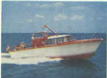
NEW OWENS "35" EXPRESS YACHT—Leaves traditional cruisers years astern! Double-planked mahogany sides and bottom, teak decks and cockpit floor, bow pulpit, full yacht railings. Two cabin plans, each sleeping 6. Incomparable performance with twin 200 h.p. Flagship Marine V8 engines. $17,795 F.O.B. Baltimore. Trade and terms.
